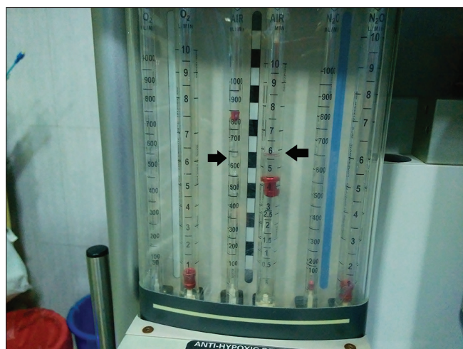
Figure 1: Markers indicating the water level present in Thrope's tube (air column) of workstation
